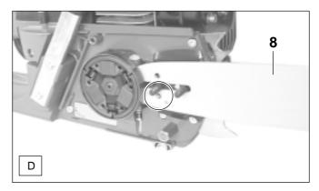
Position the guide bar (D/8). Make sure that the pin (C/7) of the chain tightener is in the hole (circled) on the guide bar.
